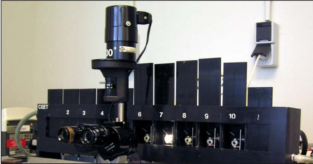
Observation of corneal effects with the slit-lamp microscope
